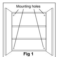
3. Hold the cabinet against the wall and align the holes in the back of the cabinet with the wall plugs. Insert the mounting screws through the holes in the back of the cabinet and screw into the wall plugs.
